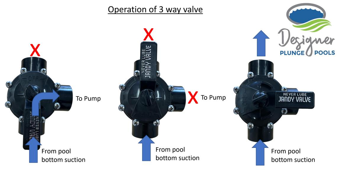
Normal mode water flowing to pump from pool Closed to block water from pool to allow filter removal and clean All open mode to drain excess water from the pool
